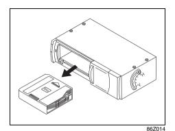
2) Press the eject button on the CD changer and remove the magazine.
